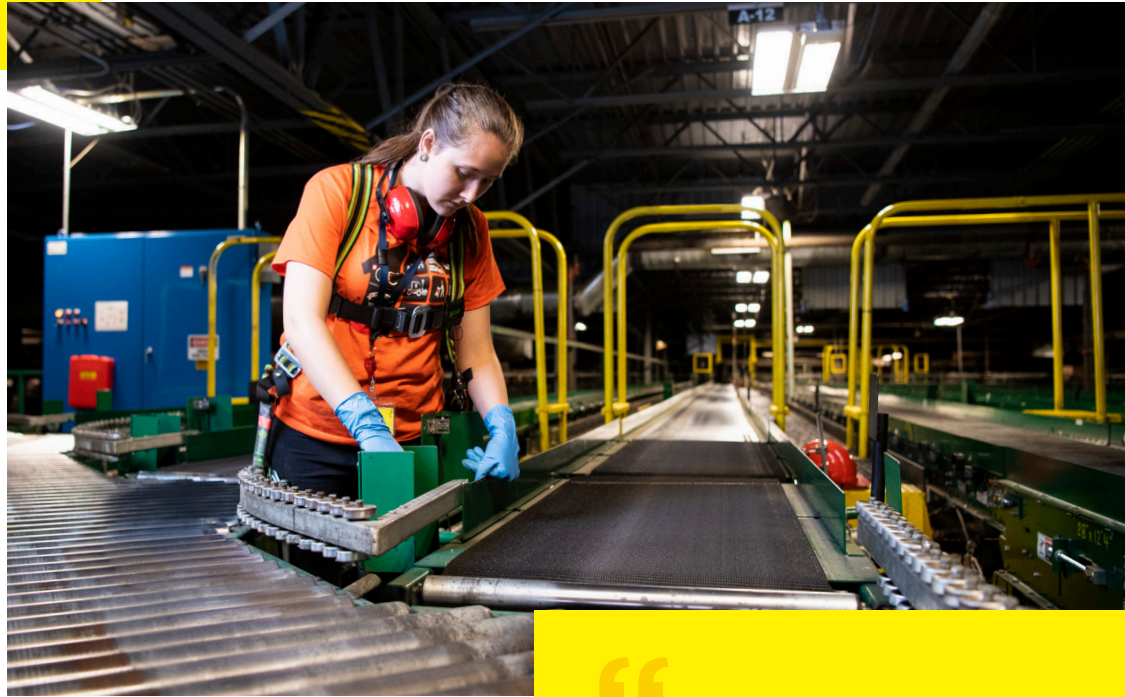
Savanna Matson inspects the conveyor belts that feed 13 miles of conveyers in the Orlando Walgreens distribution center where she works.
